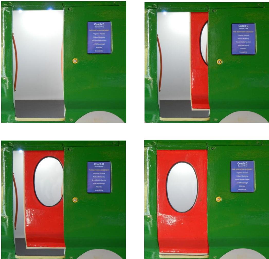
The door opens behind a large static non-scrolling destination display to give clear quick information about where you can travel to if you enter that door: especially important if trains divide en route.
