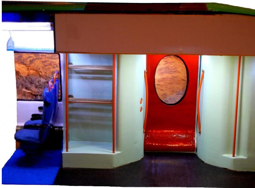
The door is 1.0m wide: enough for someone carrying a suitcase in each hand to enter or leave easily. Circulation space near the door and step-free access should speed up loading and unloading significantly, especially as the remotest seats are nearer a door than in a conventional design.
