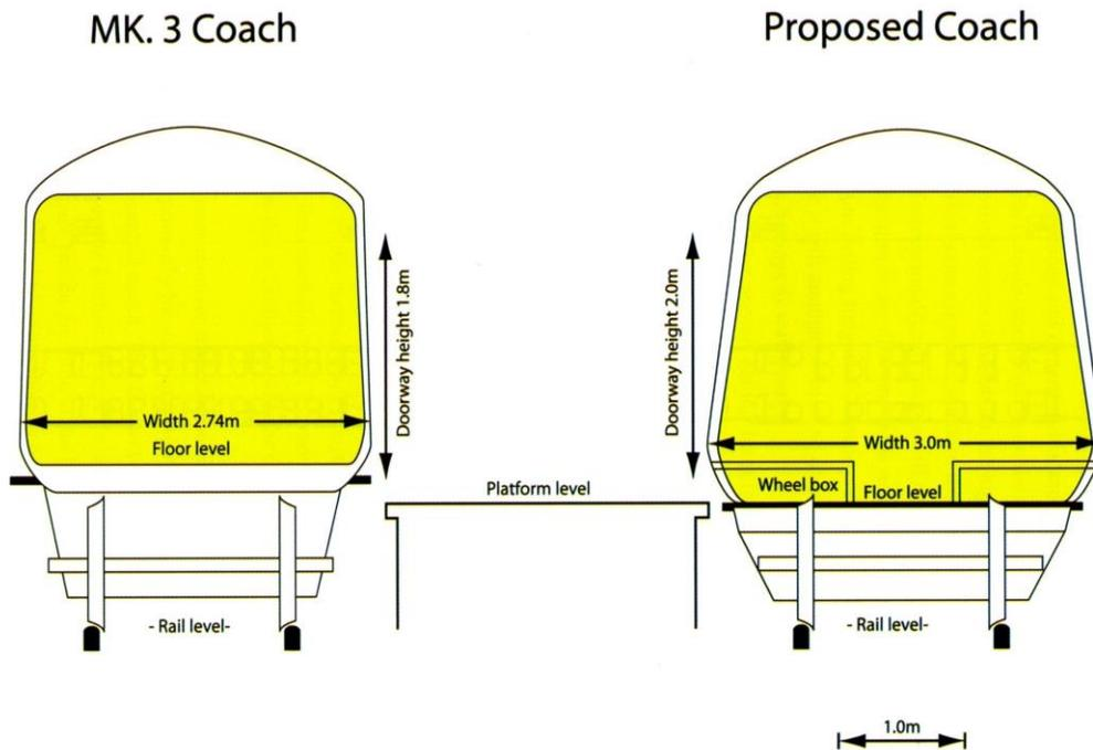
The vehicle height is the same as usual, and it conforms to the existing tolerances for 'almost anywhere' route availability below platform level and a short distance above it, allowing for variations in platform height and dynamic suspension movements. Also at or near roof level the profile is more or less the same as usual. Between those areas, however, there is a 'bulge' in the critical position between seat and shoulder level to get additional width. Just how much extra width can you get?
